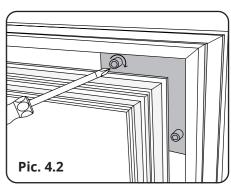
L-shaped connectors are inserted 2 pieces into each corner joint (one on each side). Then insert the screws into the l-shaped connectors and tighten them until they stop (pic. 4.2.)
