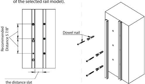
3. Fix the mounting plate measu ring with a level.
